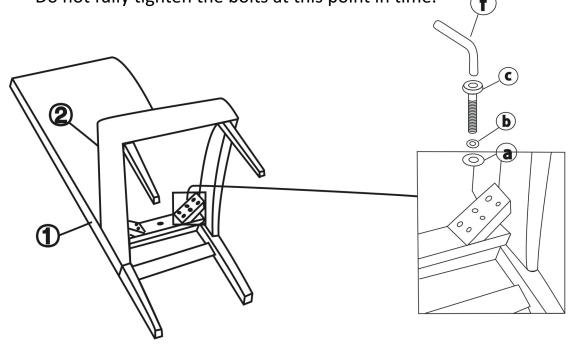
**STEP4** Carefully turn the chair over, and put the chair on the floor. Tighten each loose bolt a little at a time while marking sure the chair remains level. Repeat until all loose bolts are fully tight.
