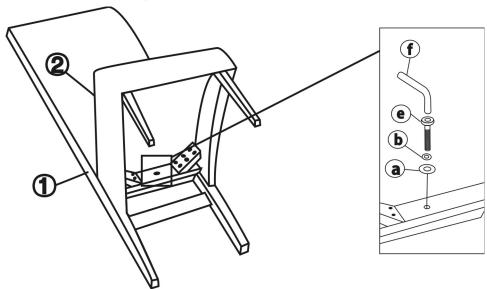
STEP3 Assemble bolts(c), spring washer(b) and flat washer(a) through each corner block of the seat (2) to the back frame.
